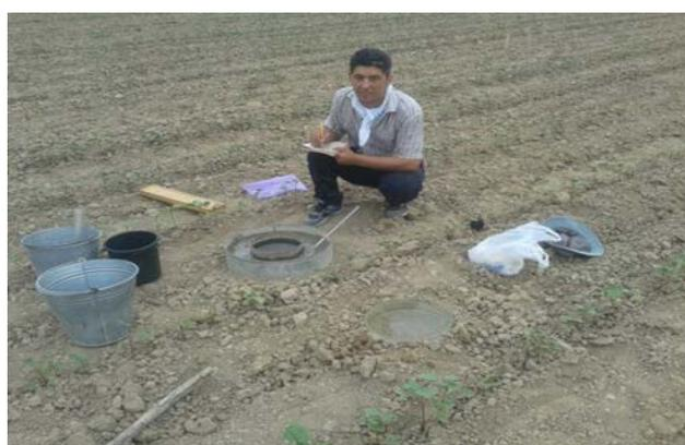
Fig. 2. Measurement of water permeability
