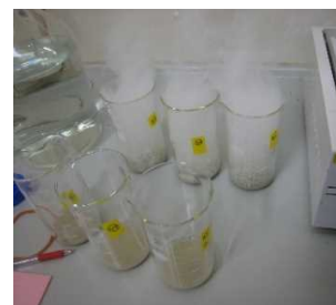
図-1 過酸化水素水（ H_2O_2 30%）による強制酸化 Forced oxidation with hydrogen peroxide solution
