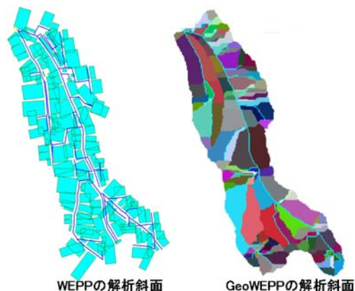
Fig.2 WEPPとGeoWEPPの解析斜面 Analysis slopes of WEPP and GeoWEPP
