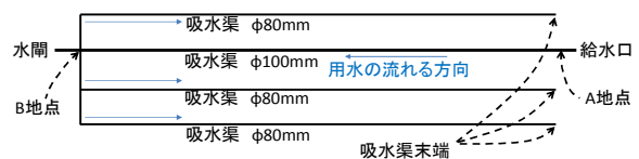
Fig. 2 調査範囲の暗渠配置 Layout of the underdrains at the surveyed area
