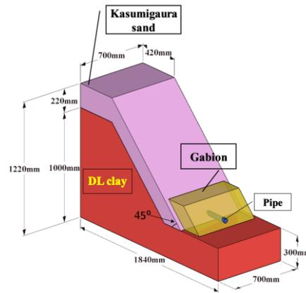
Fig. 1. Experiment slope model.
