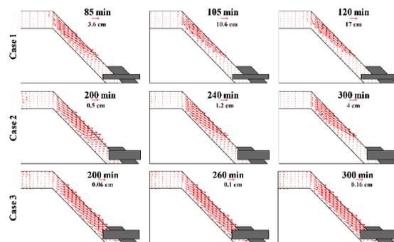
Fig. 5. Displacement vectors due to rainfall.
