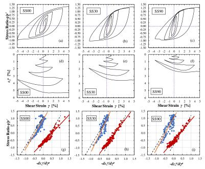
Fig. 1. (a - c) Stress-strain relationship, (d - f) Volume change behavior, (g - i) Stress-dilatancy relationship for increasing shear strain amplitude
