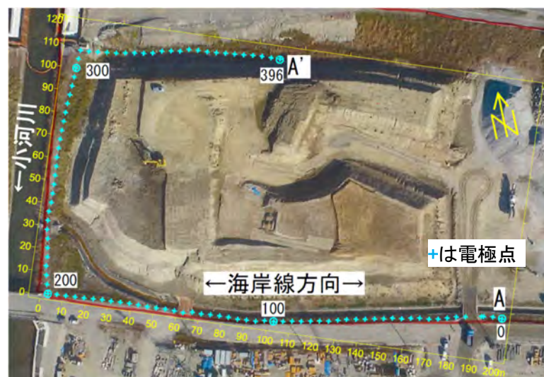
図 1 測線配置図 Fig.1 Layout of the survey line
