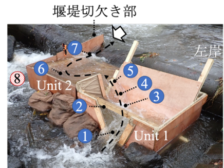
Fig. 2 水深・流速測点 Measurement points of flow velocity and water depth
