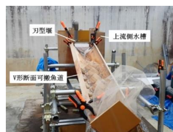
Fig.2 室内実験装置 The fishway used in the laboratory experiment
