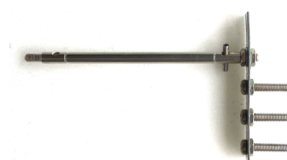
Photo 1 土壌攪乱用のツメ Experimental equipment for soil disturbance
