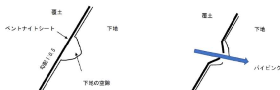
図2 GCLの下地空隙の問題 Damage to GCL due to uneven ground
