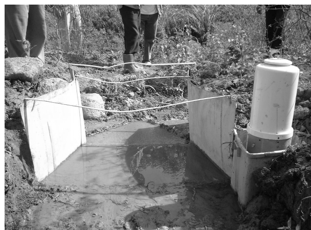
Fig. 2 The Parshall flume used in the experiment.
