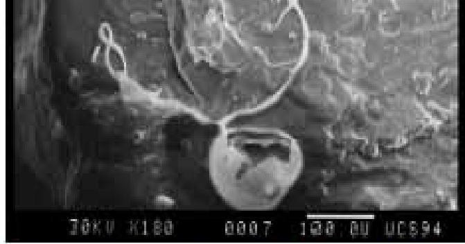
Fig. 3. Hydrophobic organic coating on a previously hydrophilic sand grain formed during an experimental burn of Eucalyptus globulus litter over dry, washed sand (SEM image, 180× magnification).
