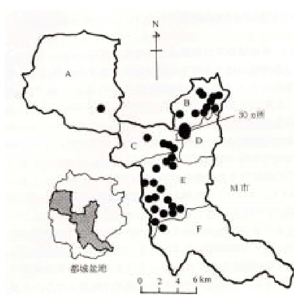
Fig.2 Distribution of measurement points where NO 3 -N concentration exceeded 10mg/L (Toyomitsu et. al., 2003)
