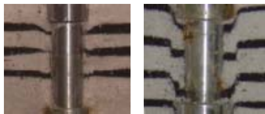
(a) p7_3 (b) p5_5 Photo 1 载荷後の地盤内挙動 Ground behavior after loading
