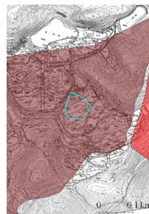
Fig.2 地すべり土塊と地形図 Slide geometry and topographical map
