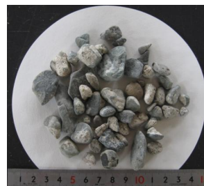
写真-2 再生骨材 M Recycle aggregate
