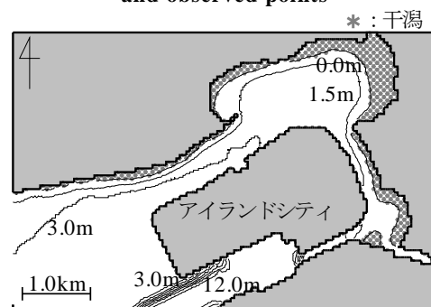
Fig.4 干潟の再現性(エッジタイプ) Simulated result of tidal flat generation, Edge type
