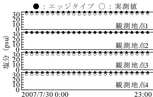
Fig.6 塩分の再現性, 博多湾(エッジタイプ) Comparison of calculated and observed salinity in Hakata Bay, Edge type
