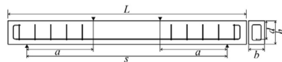
Fig. 1 試験体の形状および鉄筋配置 Shape of specimen and placement of reinforcing bar
