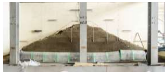
Fig. 3 開削時の底樋管外観 Appearance of outlet conduit during excavation
