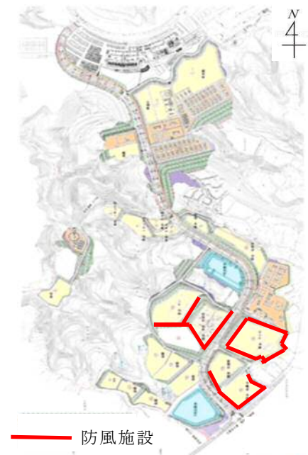
図-2 伊都農場IV工区 の防風施設 Fig.2 Windbreak facility in Ito Farm IV
