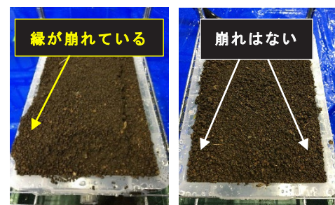
写真 3 耐雨試験後の状況 (左)未散布(右)T-2 Situation after rain resistance test(L)Not sprayed(R)T-2
