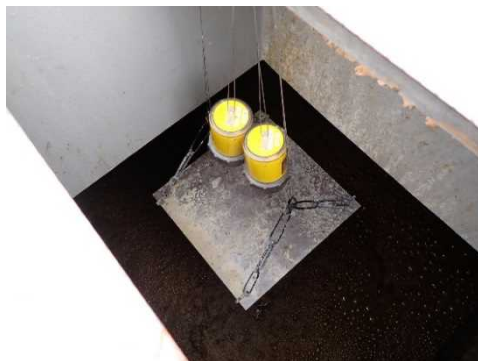
Fig.3 硫化水素濃度測定器設置状況 Installation Status of Hydrogen Sulfide Measuring Device
