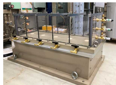
図-1 側面アクリル剛土層 Acrylic soil container
