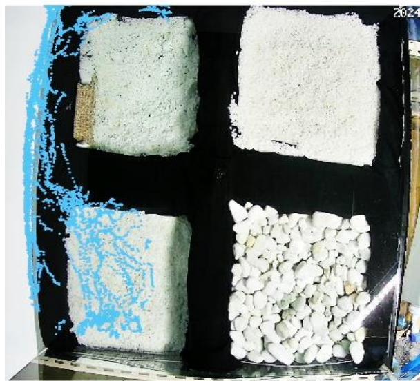
Fig. 2 StrongSort を用いたモツゴの追尾の例 Tracking swimming Pseudorasbora parva using the StrongSort algorithm
